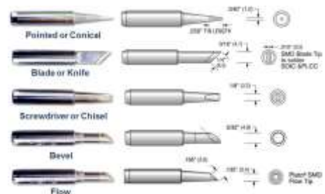
Figure 1: Tips of Soldering Iron
